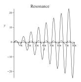
Figure: The graph of  $y = \sin(2t)$  (*dashed*) versus  $y = t \sin(2t)$  (*solid*), demonstrating the phenomenon of resonance.
