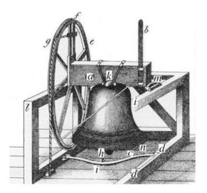
Figure : A large bell and the apparatus required to make it ring.
